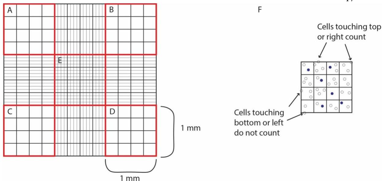
Figure 3: Cell counting with a hemacytometer.
