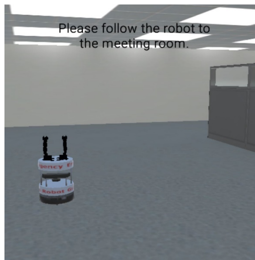
Figure 5. Robot Guidance Throughout Navigation Phase. The robot is guiding the participant in a circuitous path to the meeting room by going through another room first. Its arms appear slightly bent as it points in the direction it is moving.
