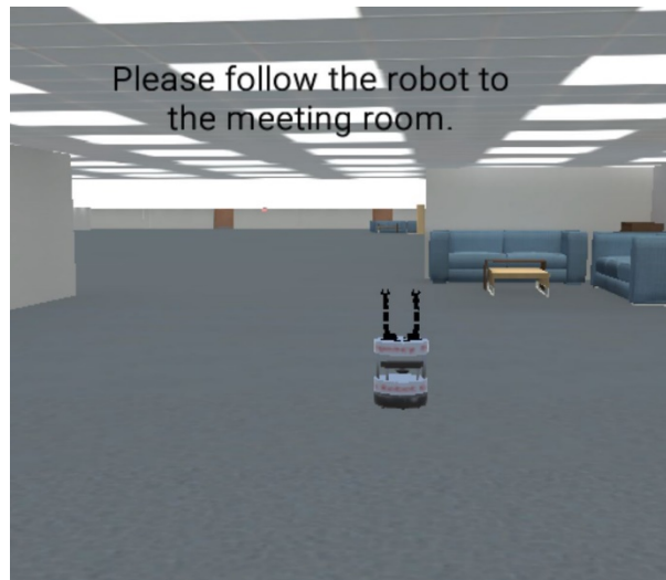
Figure 2. Evacuation Robot in Simulation Environment. This is the opening image of the main simulation environment and how the robot appears to a user. Its arms wave in the direction it is moving in.
