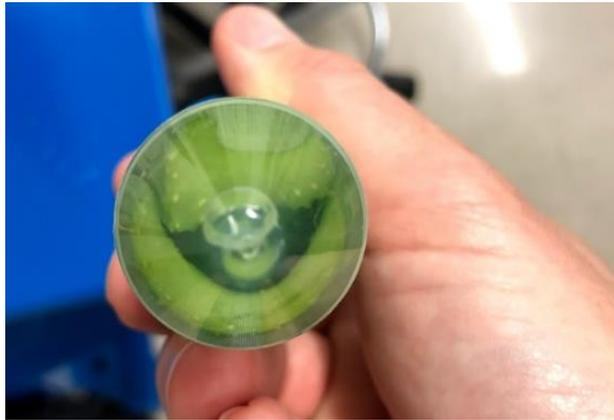
Figure 13: Two celery enclosed in a tube filled with water to observe the deformations that occurred during the mechanical test. The tube is filled with two pieces of celery to prevent the samples from moving during the scan.
